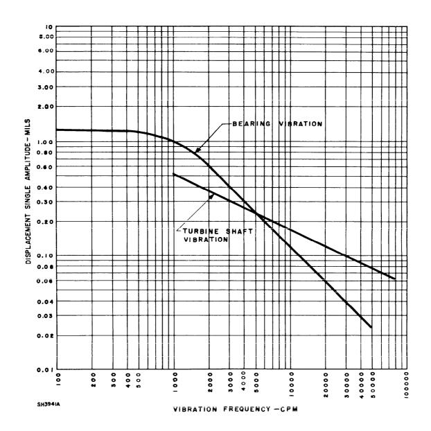
Figure 2 - Maximum allowable vibration, type II.
