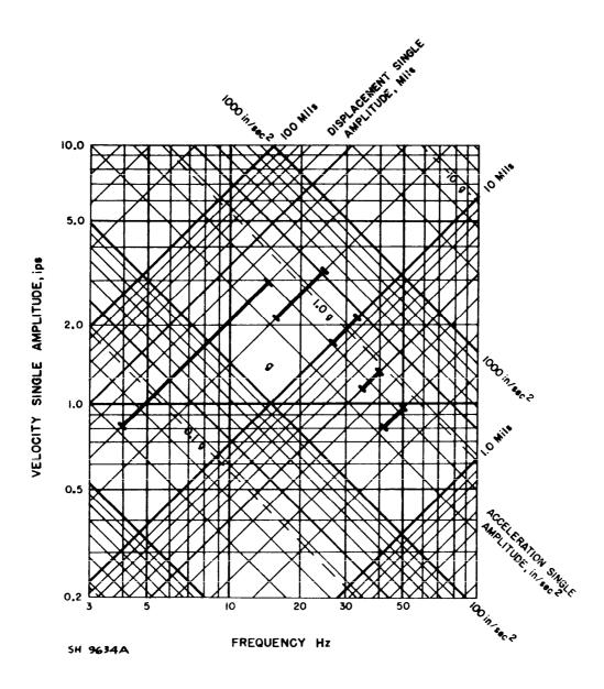
Figure 1 - Type I environmental vibration limits (graphical presentation expressed in displacement, velocity and acceleration).
